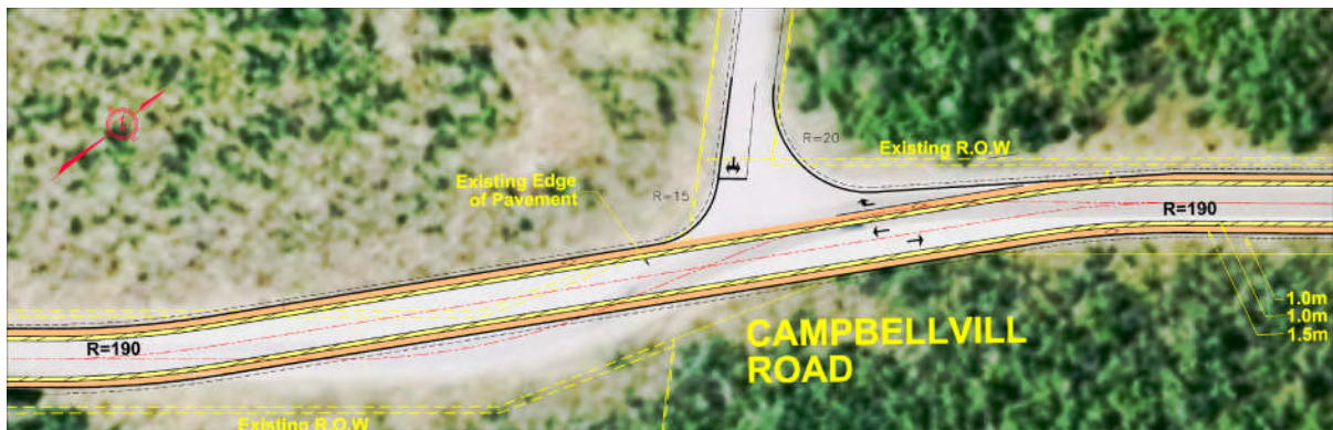
Exhibit 12-6: Horizontal Alignment Alteration on Campbellville Road
